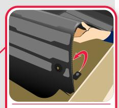
To remove the mat, place your hand underneath the mat next to the retention hook. Lift the mat up slightly and pull the mat toward the seat to unlatch the hook.
